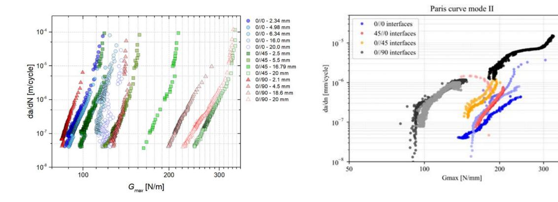
Mode I: Main effect at longer pre-cracks -> more fibre bridging
